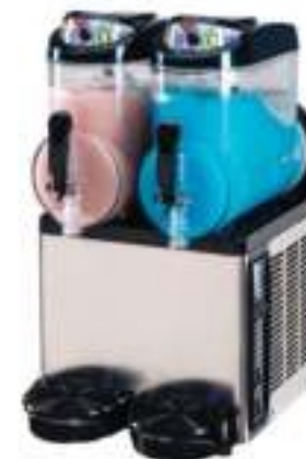
Slush Machine Cap.: 12Ltrs. × 2 Size: 430×530×800mm Power: 890W
