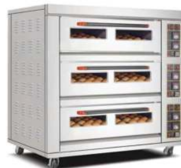
3 Deck 9 Tray, EBO 39 Dimension: 1660×820×1530mm Chamber: 1300×640×215mm Power: 25.2Kw, 380v
